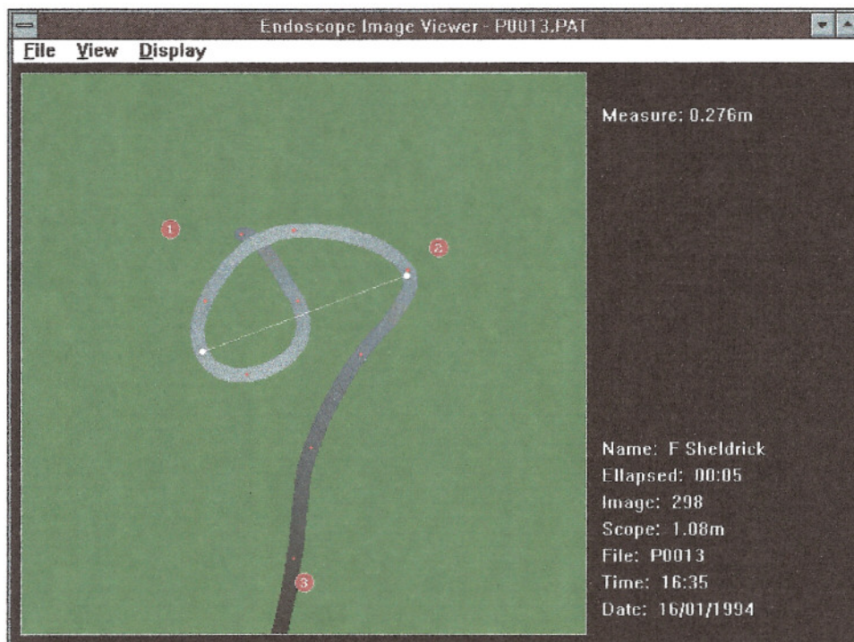
Fig 10.3: ENDOVIEW - a program for viewing the images obtained during a colonoscopy. Image shows a gamma loop forming in the transverse colon. The red dots on the endoscope indicate the position of the sensors. The white line across the image is a 3D ruler.
